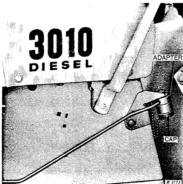
Fig. 10-10-3—Cold Weather Starting Fluid Adapter
